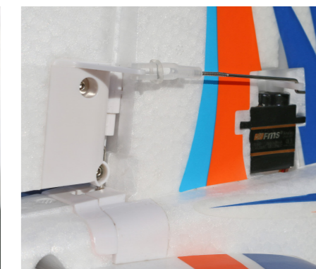
The rudder horn plate also clamps the tail wheel leg or interchangeable water rudder.
