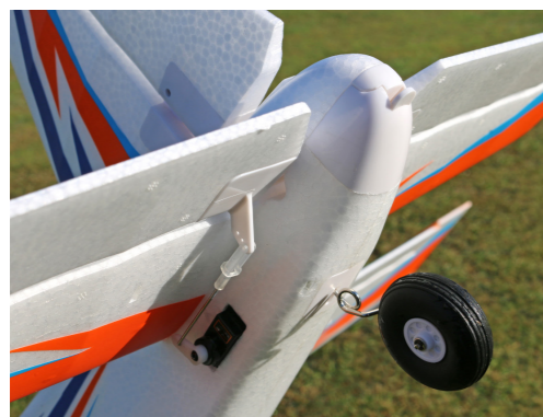
It's all good back here. That little plastic tab at the back end is pushed up to release the tailplane and slide it out.
