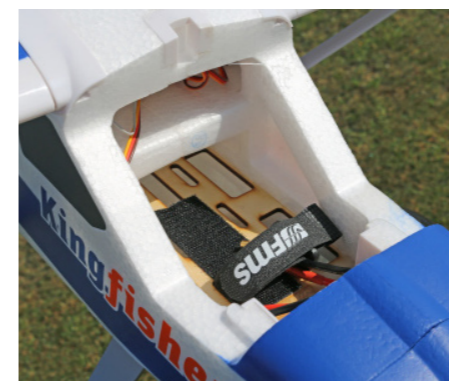
Plenty of room under the canopy for a 3S 2200mAh LiPo along with a small FPV VTx battery.
