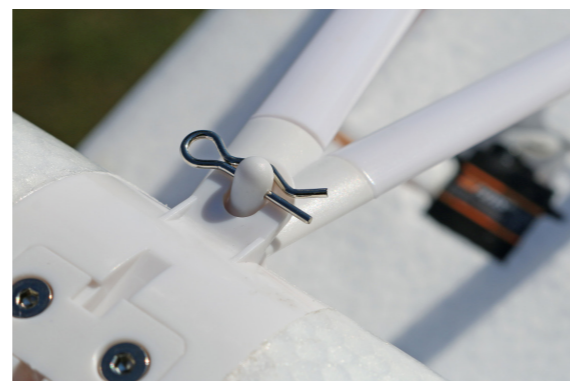
The wing struts are quick-release thanks to R-clip retaining pins.
